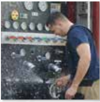
A Thornton engineer manages water pressure and flow across multiple active hose lines.
