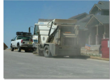
Photograph SM-7. A street sweeper removes sediment and potential pollutants along the curb line at a construction site. Photo courtesy of Tom Geis.
