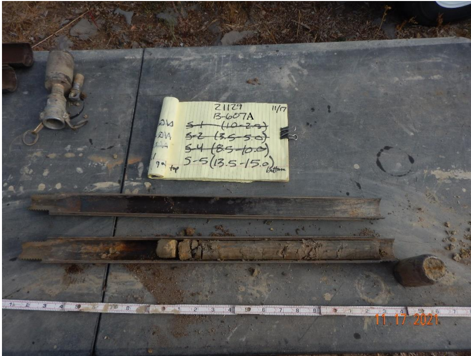
Photograph 7: B-607A S-5 from 13.5 to 15.0 feet bgs. Typical split spoon sample of Denver Formation classified as moderately to intensely weathered claystone.
