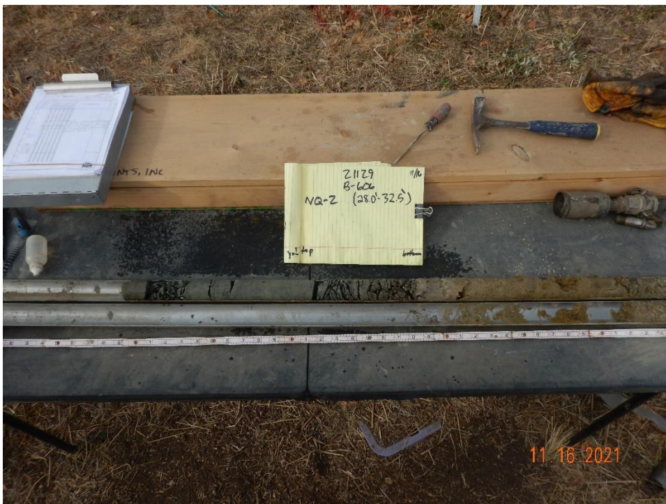
Photograph 8: B-606 NQ-2 from 28.0 to 32.5 feet bgs. Typical NQ core run of Denver Formation classified as slightly to intensely weathered claystone.
