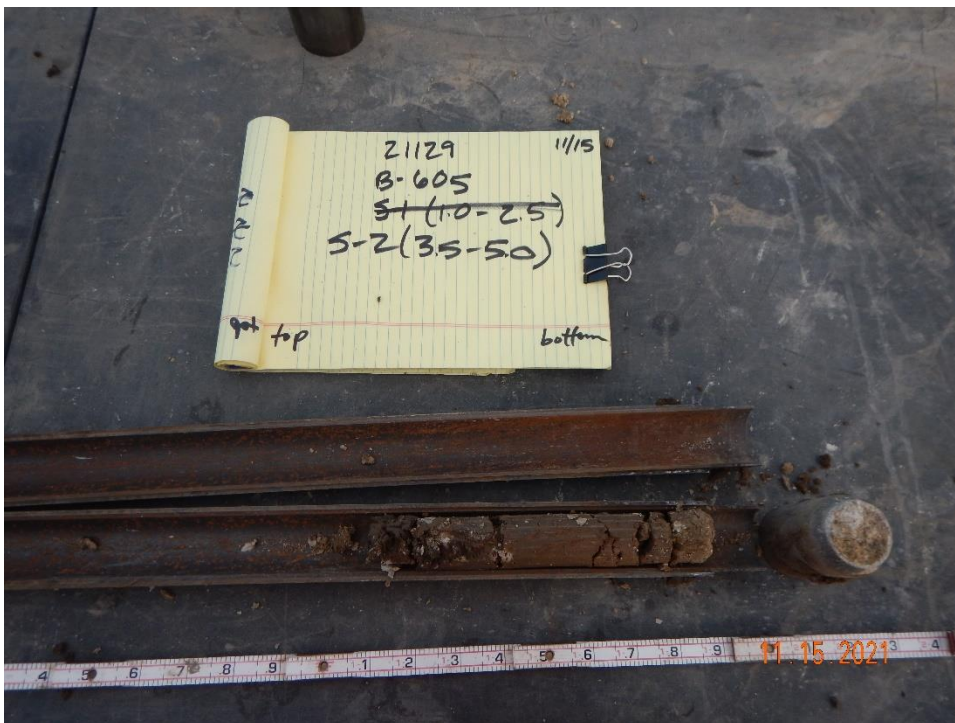
Photograph 4: B-605 S-2 from 3.5 to 5.0 feet bgs. Typical split spoon sample of fill classified as fat clay.
