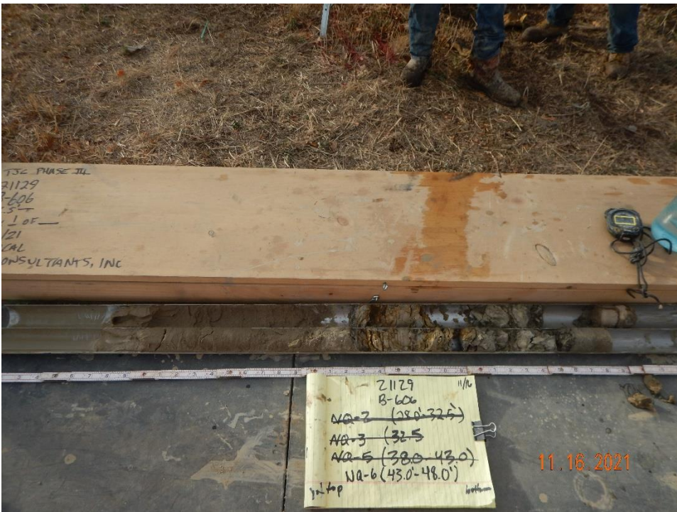
Photograph 10: B-606 NQ-6 from 43.0 to 48.0 feet bgs. Typical NQ core run of Denver Formation classified as moderately to very intensely weathered claystone from 43.0 to 44.9 feet and 46.1 to 48.0 feet and fresh to slightly weathered clayey sandstone from 44.9 to 46.1 feet.
