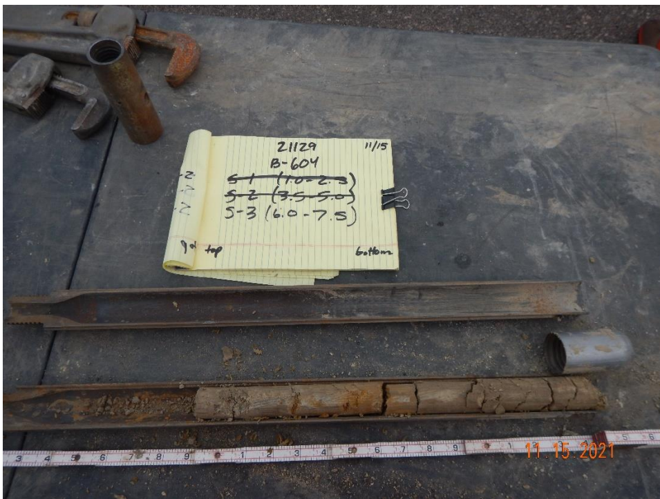
Photograph 6: B-604 S-3 from 6.0 to 7.5 feet bgs. Typical split spoon of Denver Formation classified as intensely to very intensely weathered claystone.
