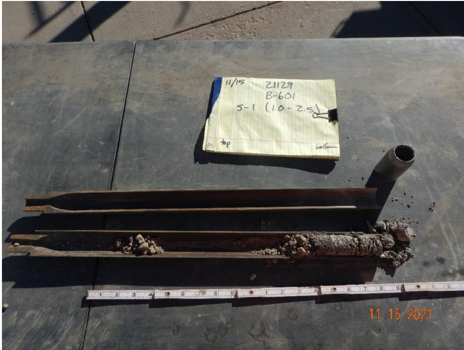
Photograph 1: B-601 S-1 from 1.0 to 2.5 feet below ground surface (bgs). Typical split spoon sample of asphalt pavement.
