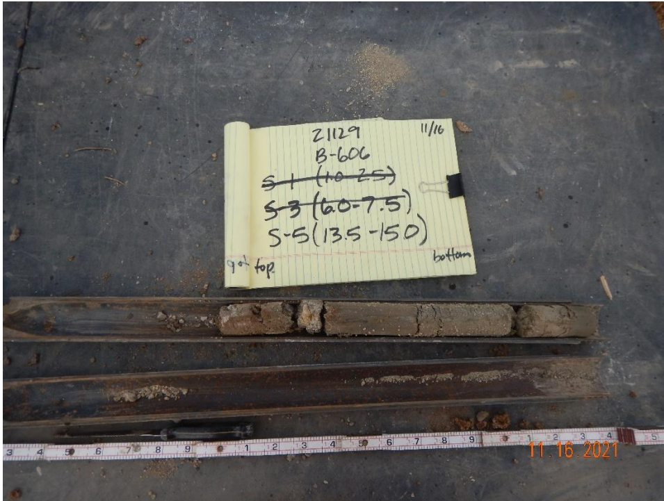
Photograph 3: B-606 S-5 from 13.5 to 15.0 feet bgs. Typical split spoon sample of fill classified as fat clay with sand.
