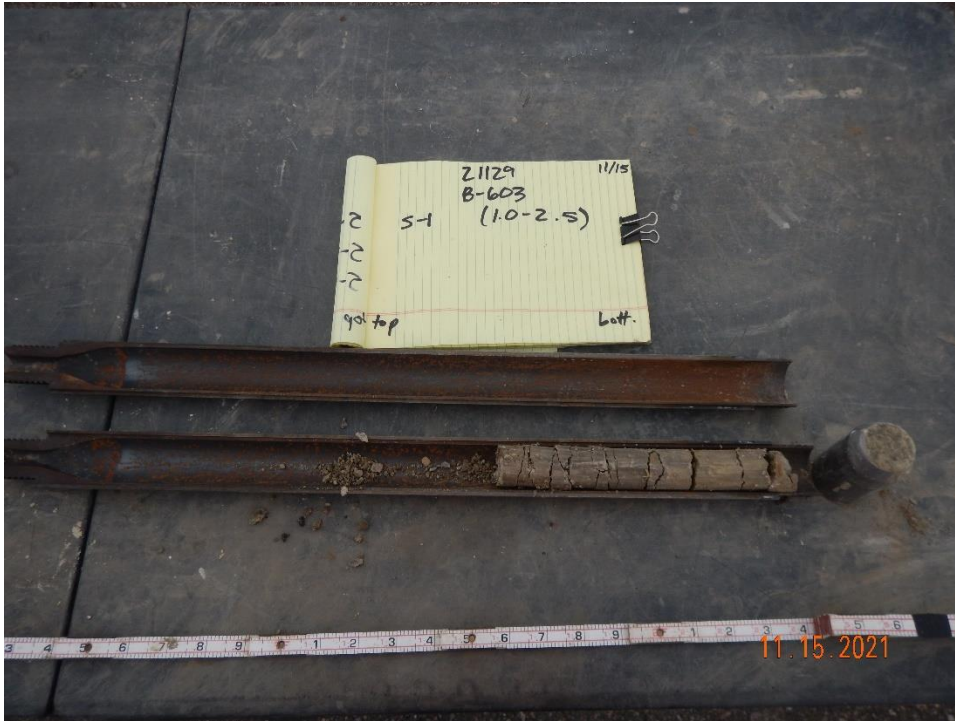
Photograph 5: B-603 S-1 from 1.0 to 2.5 feet bgs. Typical split spoon sample of fill classified as lean clay.
