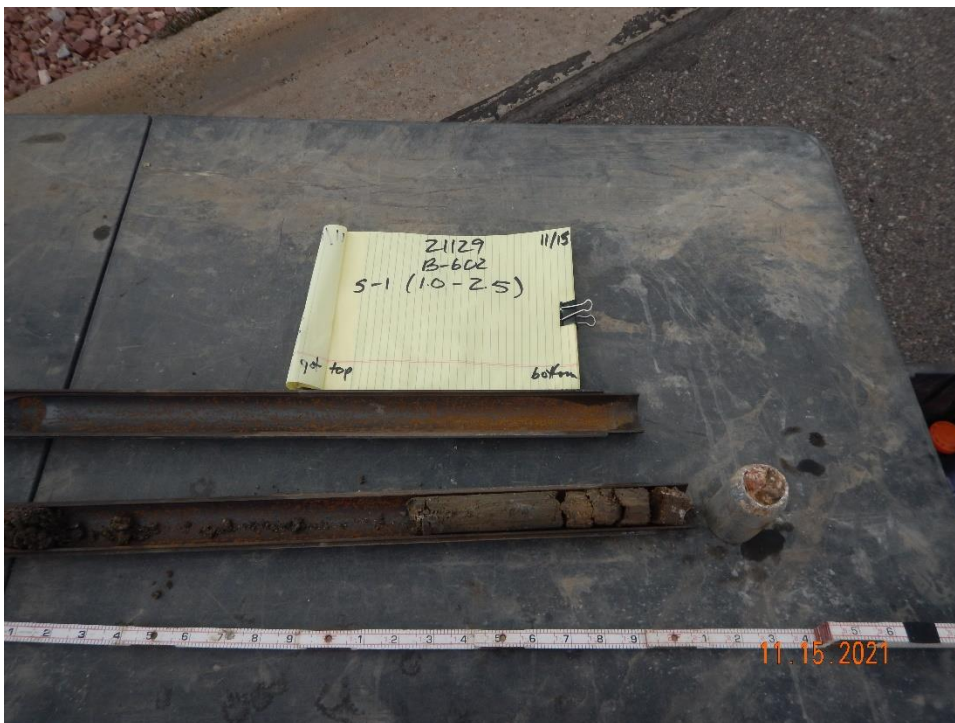
Photograph 2: B-602 S-1 from 1.0 to 2.5 feet bgs. Typical split spoon sample of fill classified as sandy fat clay.
