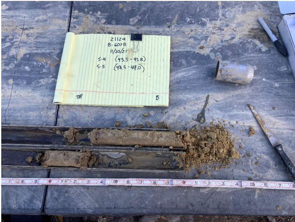
Photograph 12: B-607B S-5 from 48.5 to 49.0 feet bgs. Typical split spoon of Denver Formation classified as moderately to intensely weathered sandstone.
